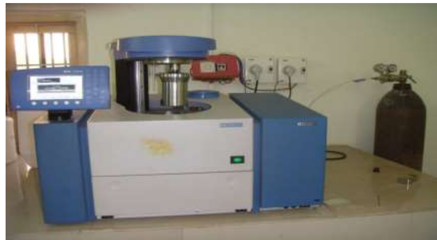
IKA Bomb Calorimeter for testing Calorific Value
